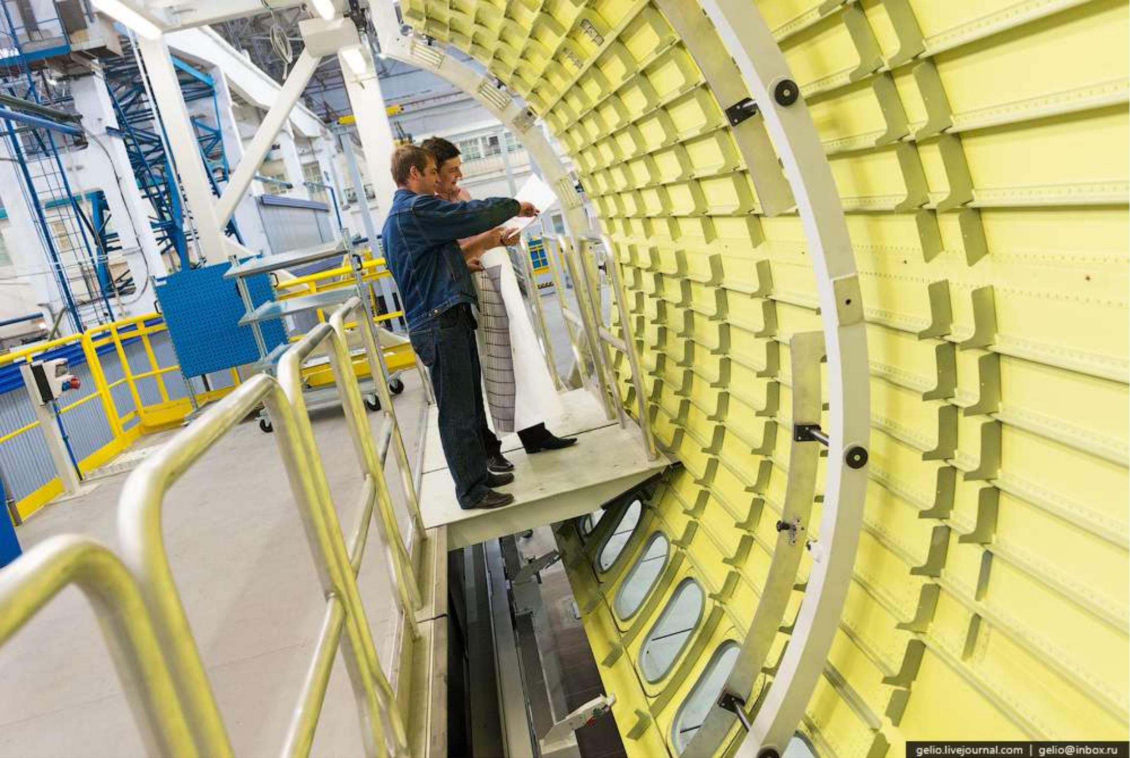
Fuselage Panel Assembling
