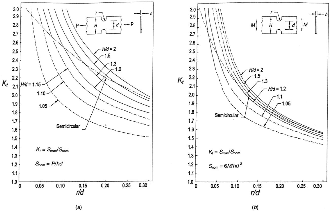
Fig 9.4 Stress concentrations factors for a flat bar with opposite U-shaped notches (a)Tension, (b)Bending
