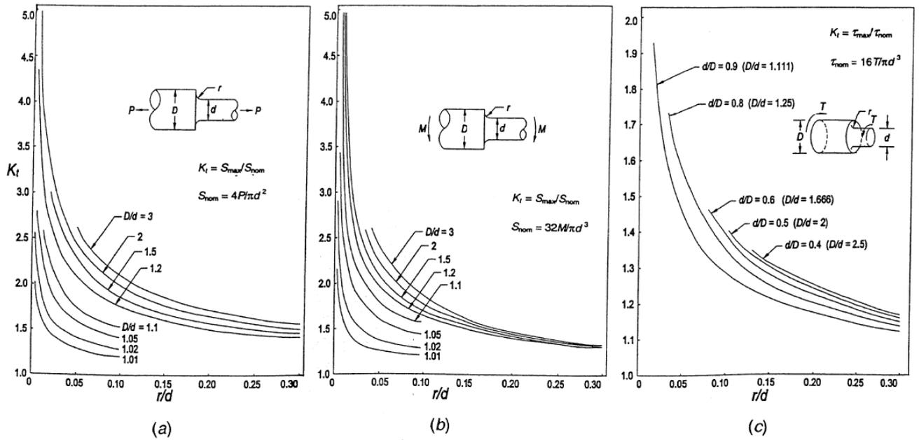
Fig 9.3 Stress concentrations factors for a stepped shaft (a)Tension, (b)Bending, (c)Torsion
