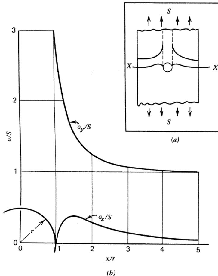
Fig. 9.2 Stress distribution along the section X-X near a hole in a wide sheet
