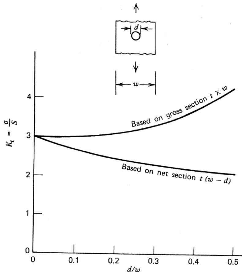
Fig. 9.1 Elastic stress concentration factor for a central circular hole in a sheet
