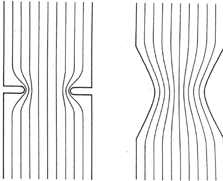
Fig. 9.5 The crowding and bending of flow lines near obstructions helps to visualize the concentration of stresses and strains near notches. The large section and the small section are the same in both cases, but the transitions are different
