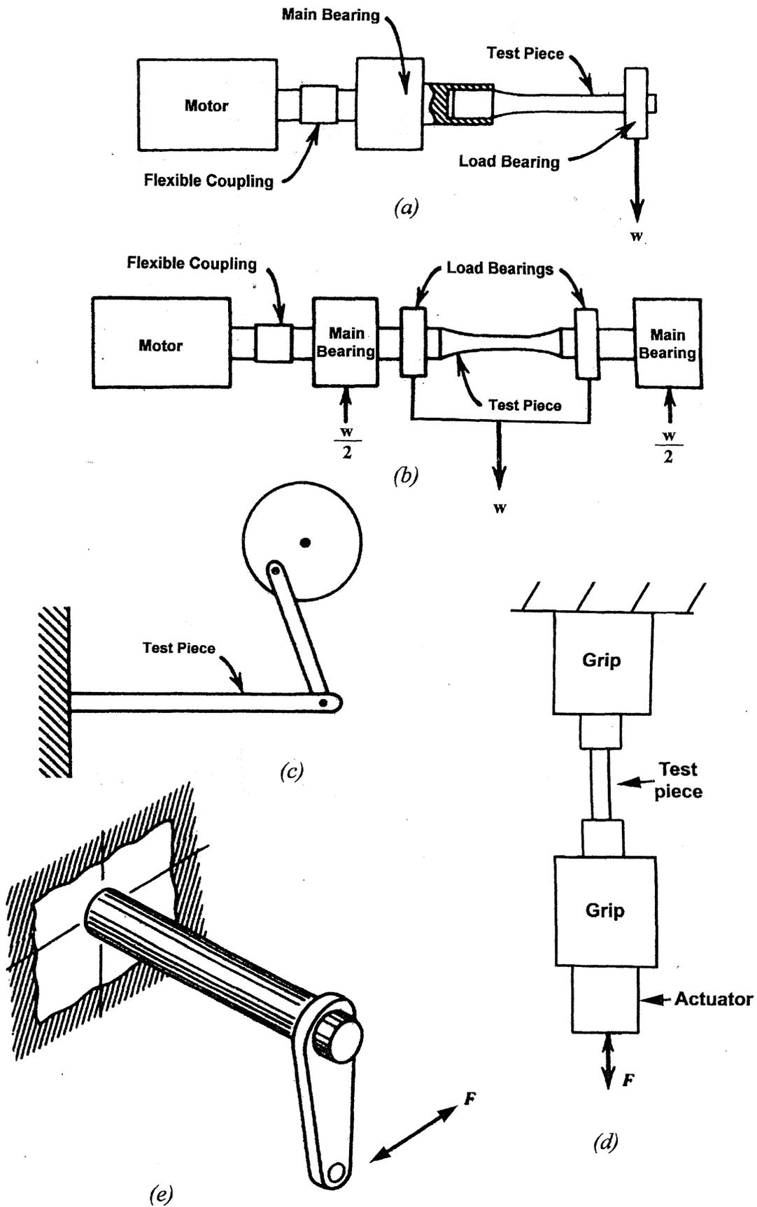
**Figure 3.** Fatigue testing machines, (a) Cantilever rotating bending, (b) Rotating pure bending, (c) Bending cantilever eccentric crank, (d) Axial loading, (e) Combined torsion and bending
