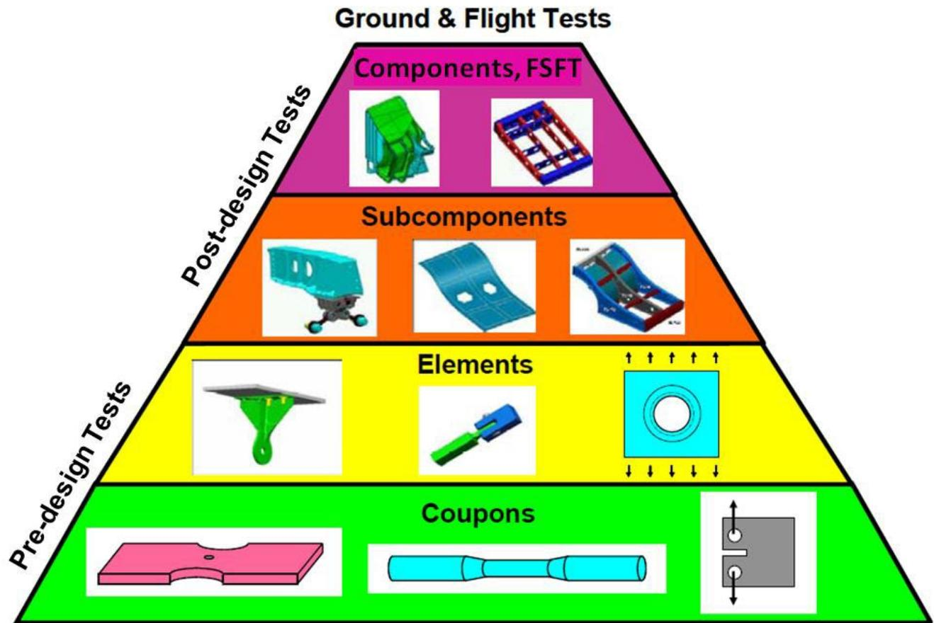
“Building Block” fatigue test approach for materials, components and structures
