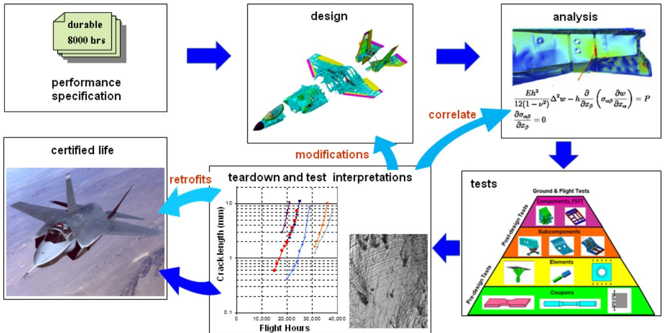
Fig. Airframe fatigue certification and the central role of fatigue testing
