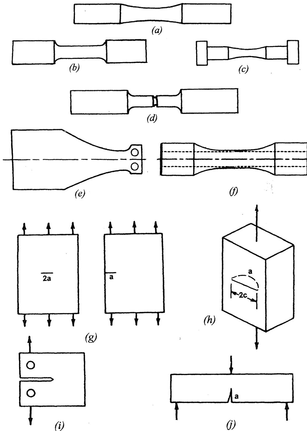
Figure 5 Fatigue test specimens. (a) Rotating bending. (b) Axial uniform. (c) Axial hourglass. (d) Axial or bending with circumferential groove. (e) Cantilever flat sheet/plate. (f) Tubular combined axial/torsion with or without internal/external pressure, (g) Axial cracked sheet/plate. (h) part-through crack, (i) Compact tension. (j) Three-point bend.
