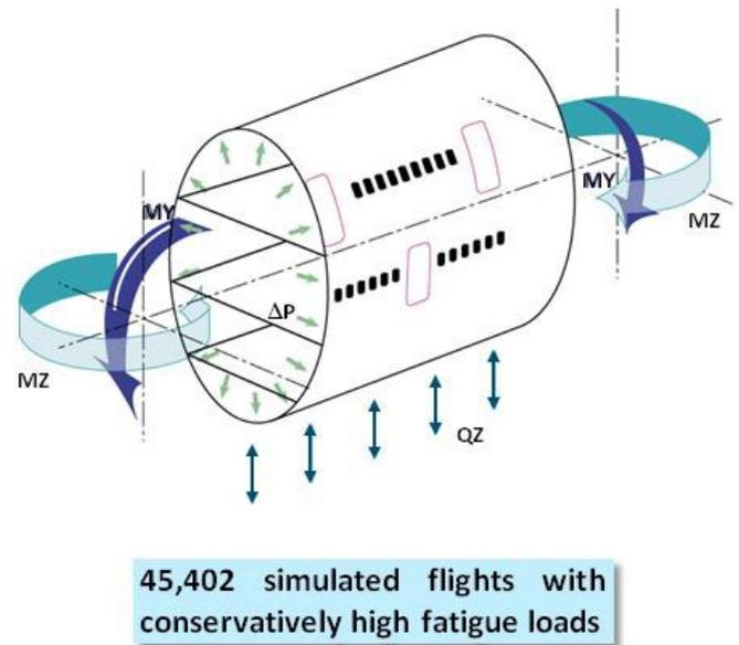
Fig. Airbus A380 full-scale fatigue test ‘specimen’, the general loading conditions, and the number of simulated flights applied during testing
