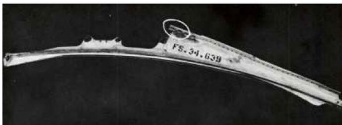
Failed door-cylinder bracket
