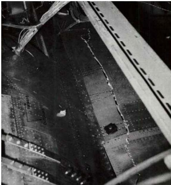
Fatigue failure of lower wing surface after spectrum loading
