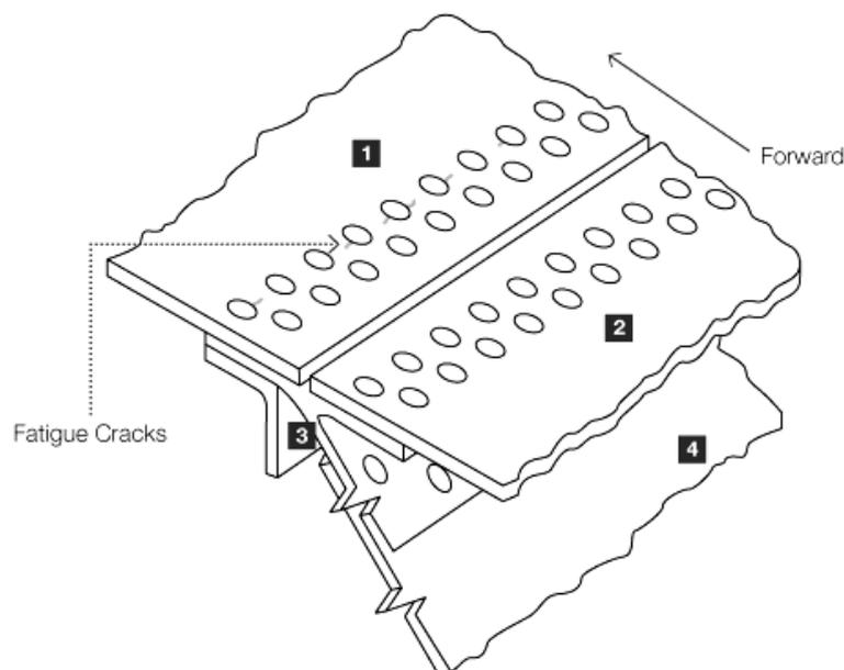
Fig.5.3. Skin attachment to the aft pressure bulkhead: 1- pressurized fuselage skin; 2 - unpressurized fuselage skin; 3 - “Y” - Tee chord; 4 – aft pressure bulkhead
