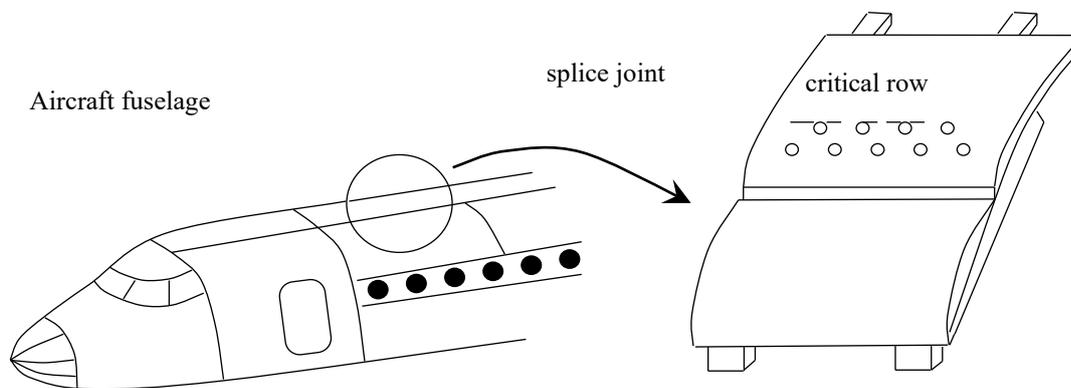
Fig.5.1. Schematic representation of MSD in an aircraft fuselage.
