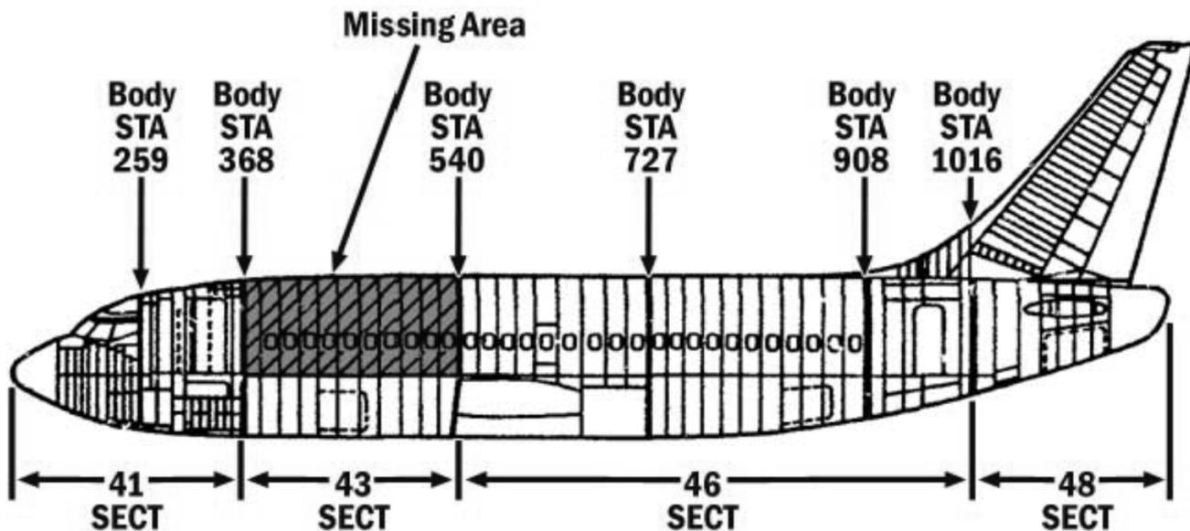
Fig.5.4. Schematics of Damage Cause to Aloha Airline Flight 243
