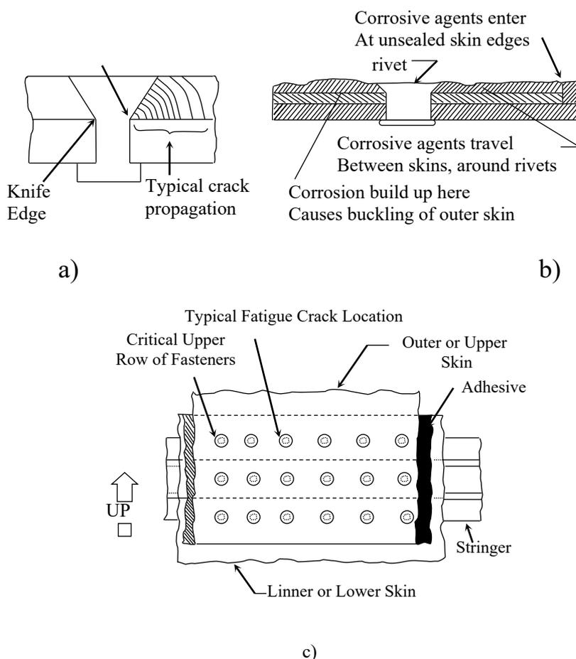
Fig.5.5. Failure of riveted structure: a) corrosion in riveted joint; b) nucleation of the crack at the “knifeknife” edges of holes; c) failure initiation in the critical upper row of fasteners
