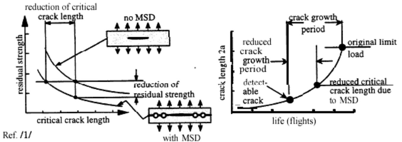
Fig.5.2. The effect of MSD on a crack.
