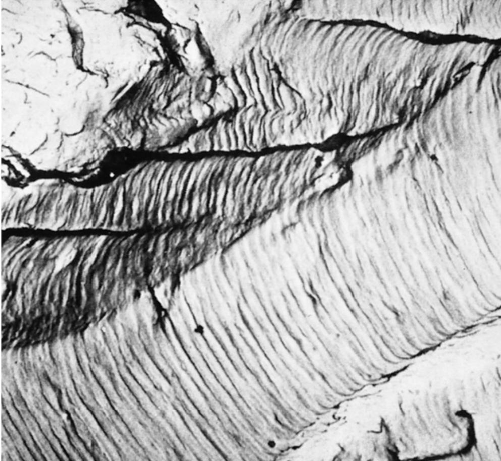
Fig.9. Striations in the stable fatigue crack growth propagation in aluminium alloy
